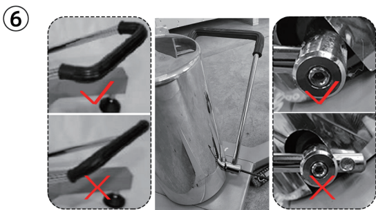
Correctly install the hydraulic foot pedal according to the diagram.
